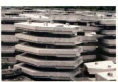
Cracked in the design of Dr Lee's walls are the hexagonal-shaped blocks of pre-cast concrete, each reinforced with steel bars to form the walls' skeletal structure.
